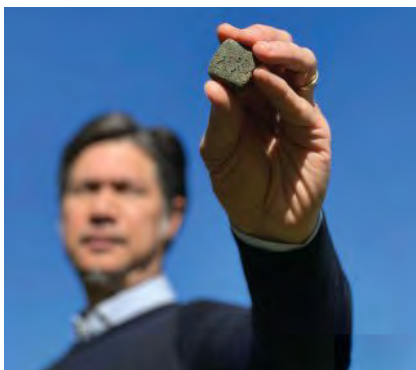
Sun rays plus conventional raw kiln feeds equals solar clinker.
