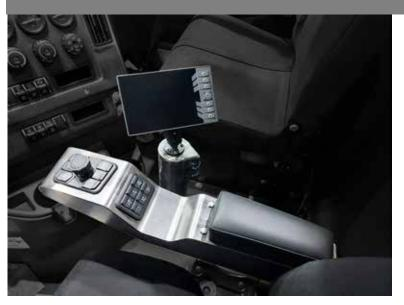
Our RESULTS controls system was developed with the driver's comfort and safety in mind. Our intuitive integration of the controls with the armrest provides the driver with access to the controls without straining themselves or holding odd positions.
