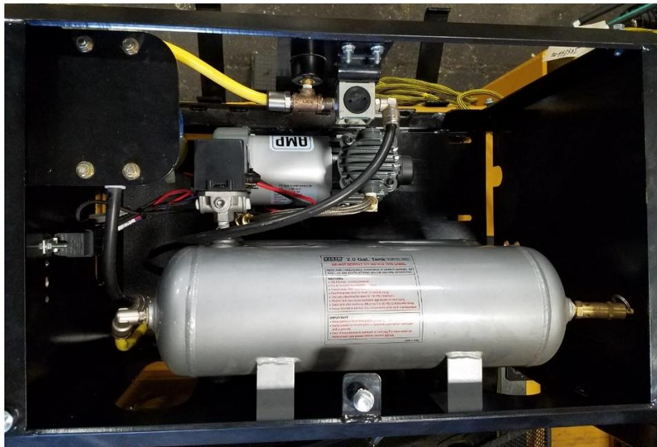
**Figure 19:** Air compressor (top view, cover off)
