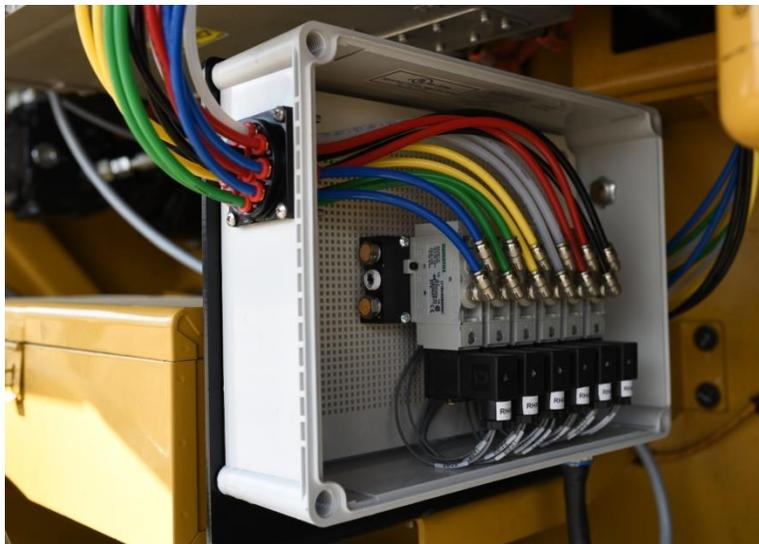
**Figure 20:** Solenoid valve manifold in its enclosure
