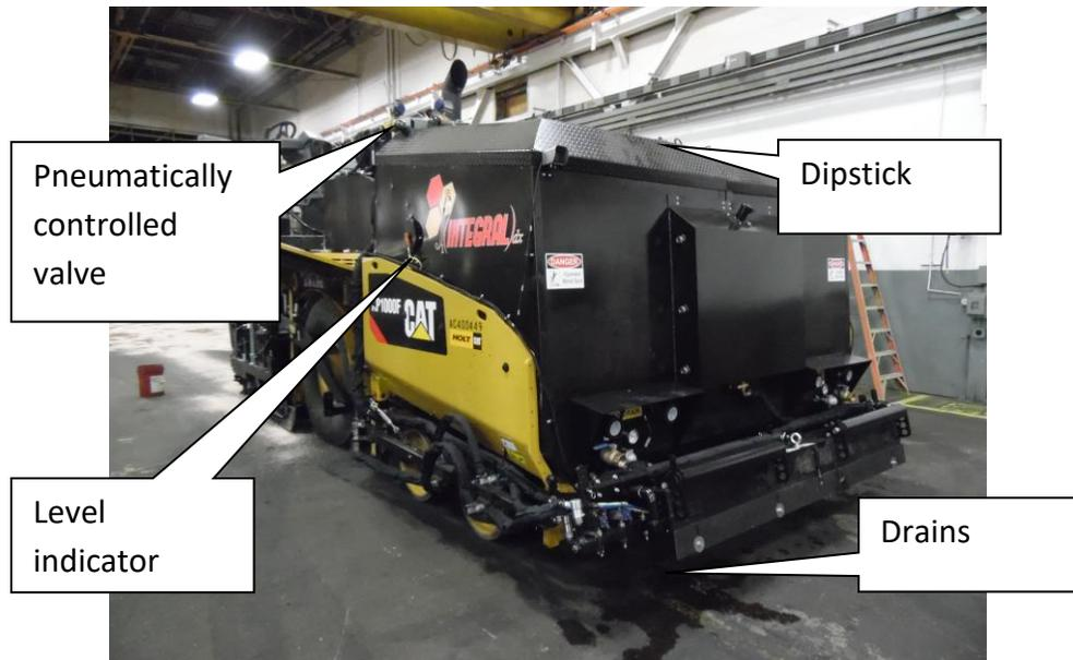
**Figure 4:** Emulsion tanks, asphalt hopper mounted
