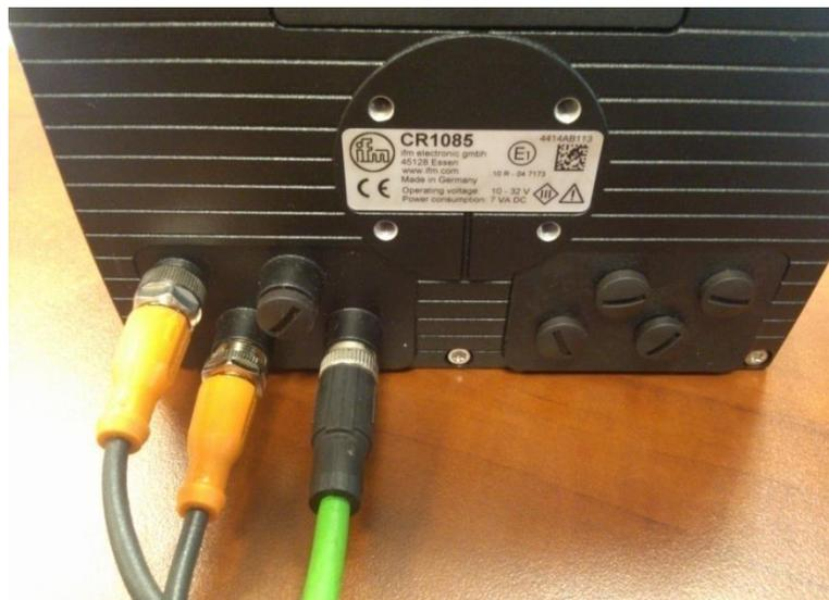
**Figure 51:** Displays screen unit back side showing the Ethernet cable connection
