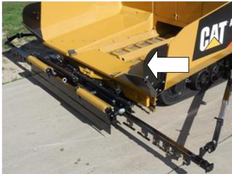
**Figure 16:** Asphalt hopper extensions
