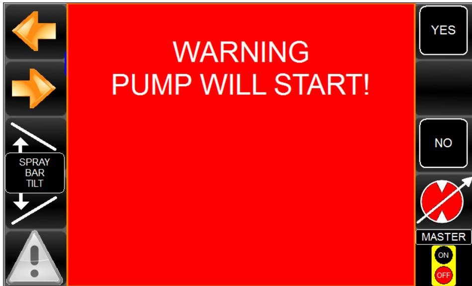
**Figure 34:** Pump will start warning screen
