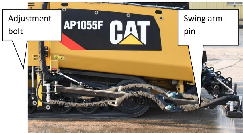
**Figure 12:** Swing arm height adjustment points
