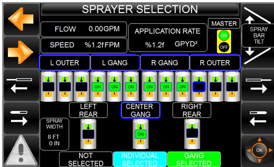
**Figure 31:** Sprayer Selection screen: some switches selected, pump on in Auto Spray, and master spray switch on
