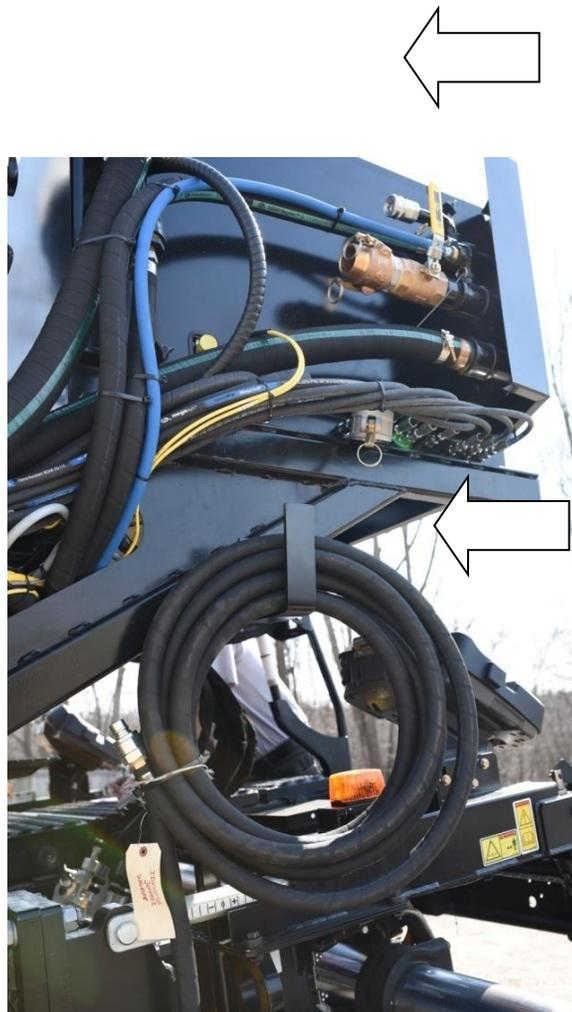
**Figure 15:** Spray wand connection and hose
