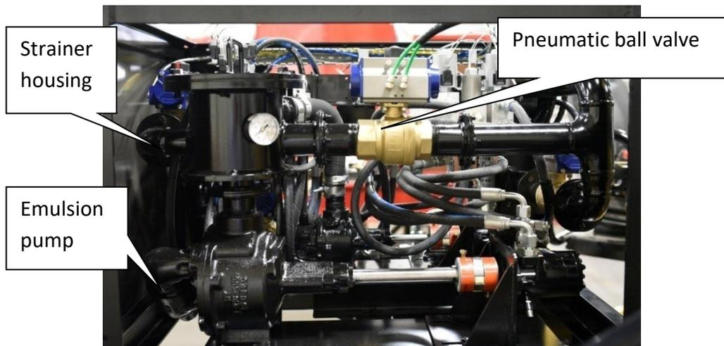
**Figure 5:** Emulsion pumping station (right-side view)
