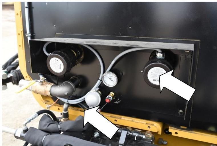
**Figure 21:** Tank heating elements and thermostat temperature sensor
