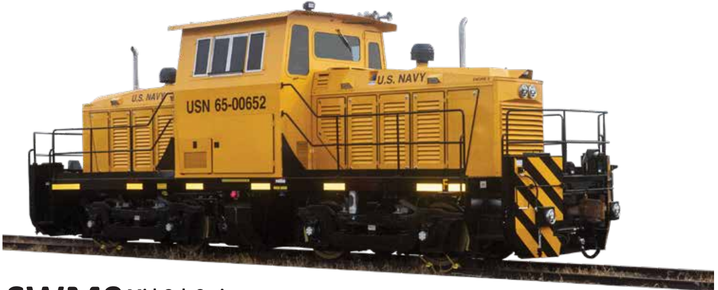
SWM9 Mid-Cab Series Switcher, Mid-mount cab 82 ton 900 hp
